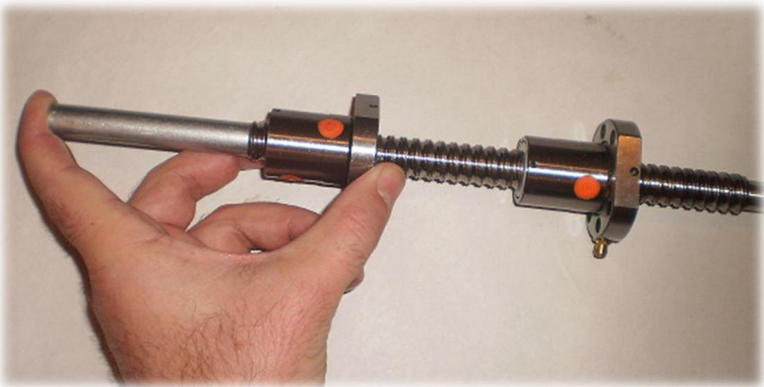
Continue turning in the same manner until a portion of the screw thread emerges from the other side. At this point, carefully remove the retainer once the ball is fully inserted on the screw.
